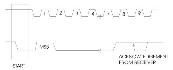
The audio processor that has been addressed has to generate an Acknowledge after receiving each byte, otherwise, the SDA Line will remain at the High Level during the ninth (9th) Clock Pulse. In this case, the master transmitter can generate the STOP Information in order to abort the transfer.
